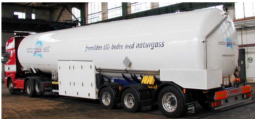
Figure 2. LNG semitrailer 56 000 liter, 7 bar MAWP
