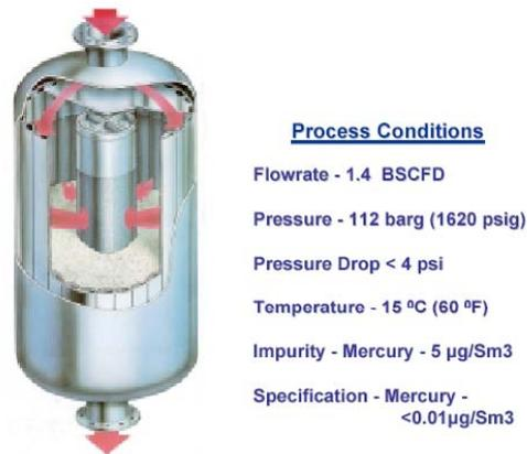
**Figure 3: Cut-away Diagram of a Radial Flow Reactor**
