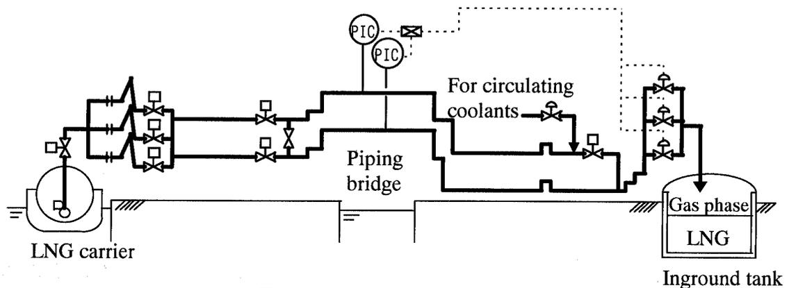
Figure 6. Flow Diagram of Receiving Piping
