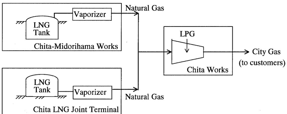
Figure 5. Gas Flow Sheet
