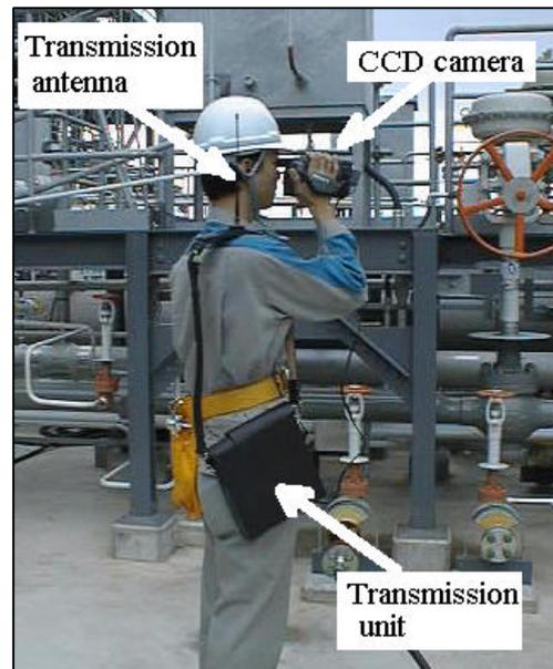
Figure 7. System Usage Conditions
